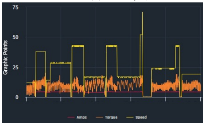
Runtime and Pump Speed Monitoring Graphic
